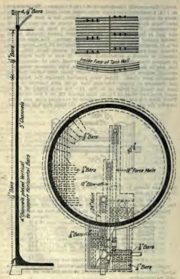
Fig. 22.—Reinforced Concrete Standpipe.
